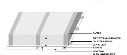
Further strips of Vapreflex® are then put in place with an overlap of not less than 50 mm, and 75 mm Aluthermo® adhesive is applied to achieve tightness.
