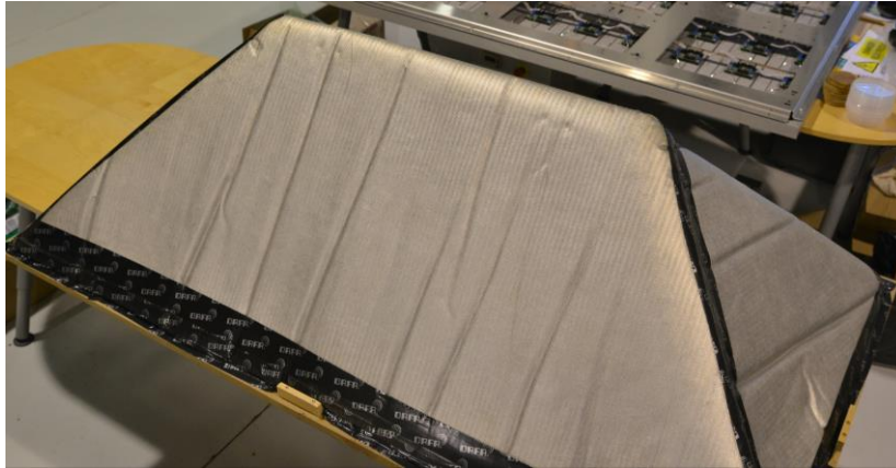
Figure 9 - Structure insulated with 1 layer of Aluthermo DENSIMA®
