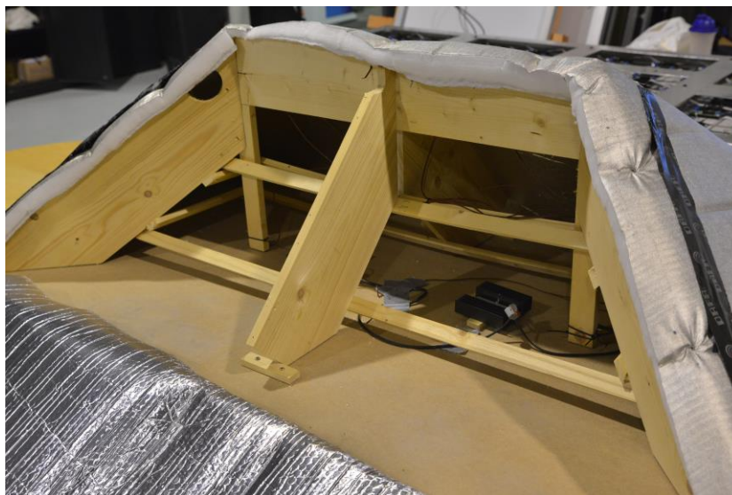
Figure 10: Inside view of structure insulated with Aluthermo DENSIMA®
