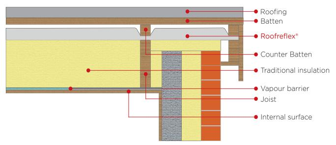
Aluthermo Roofreflex<sup>®</sup> can also be fitted draped without counterbattens (only UK market)
