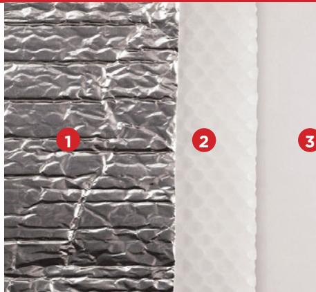
The aluminium sheets reflect thermal radiation summer and winter, while the polyester wadding core and the dry, stable air trapped in the bubble film effectively slow the transfer of energy by conduction. This thin, high-performance insulation material also offers an impermeable barrier to moisture and is vapour proof.
